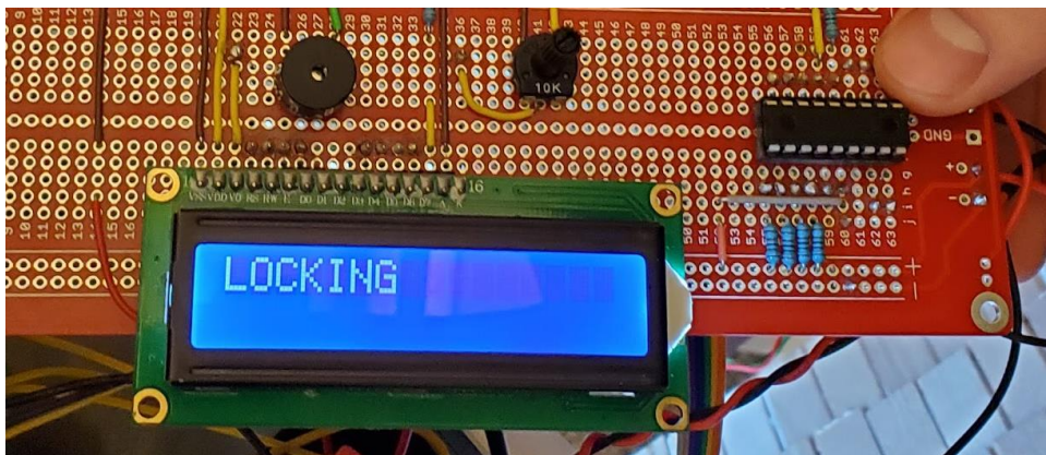
Figure 9: Example Status Display on LCD Screen
