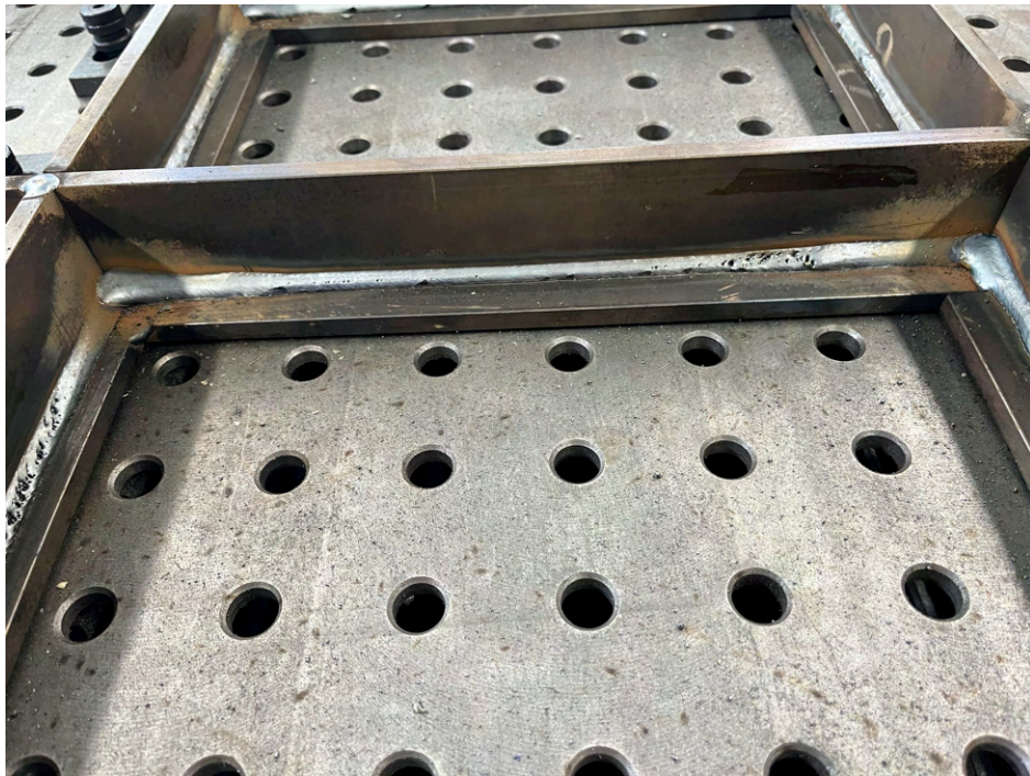
Figure 3.5: Corner to Corner Welds with Porosity
