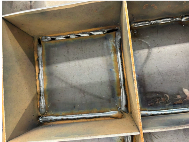
Figure A.10: Burn-through Welds of the Original \frac{1}{8} Inch thick Weld Grid
