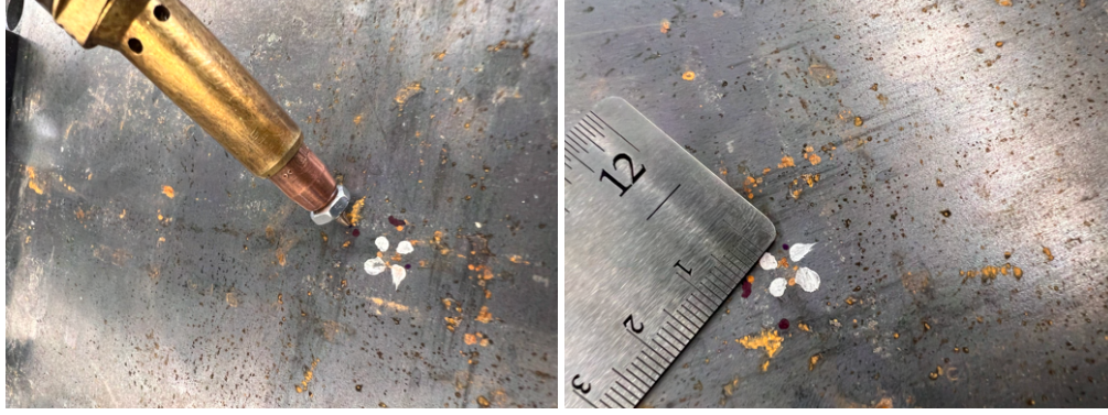
(a) TCP Error: metal tip versus white dot (b) TCP Error Measured Distance
