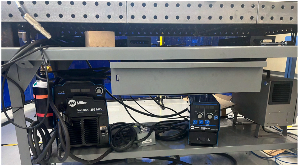
Figure B.12: Under-side of Weld Table with: Invision 352, Insight Module, S-74, and UR10e controller
