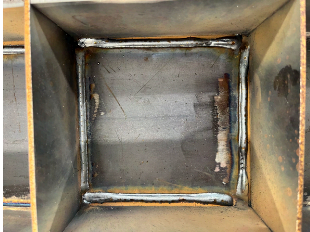
Figure A.9: Misaligned Welds of the Original \frac{1}{8} Inch Thick Weld Grid
