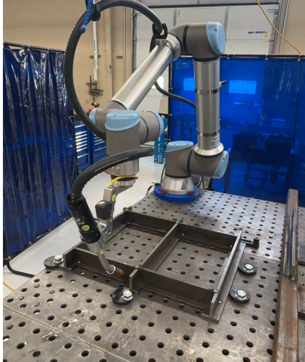
Figure 2.3: UR10e with BA1 Weld Gun with Work-Piece
